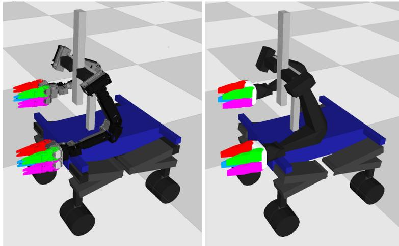
Figure 3: Left: Detailed rendering of the Momaro robot. Right: Fine collision model of the same robot to ease collision checking based on the convex hull of its limbs.
