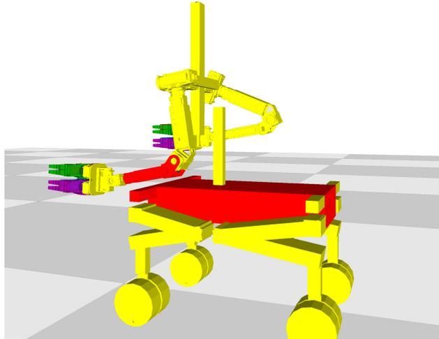
Figure 4: Rendering of the robot model for the support operator indicating close proximity between the lower left arm and the base.
