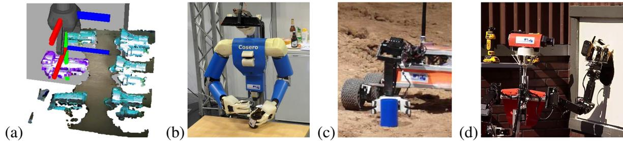
Figure 2: Example manipulation robots at University of Bonn: (a) Depalettizing with Universal Robots UR10 manipulator and Robotiq three-finger hand [31]; (b) Bottle opening with cognitive service robot Cosero [74]; (c) Grasping a water-filled mug with space robot Explorer [77]; (d) Cutting drywall with mobile manipulation robot Momaro [61].
