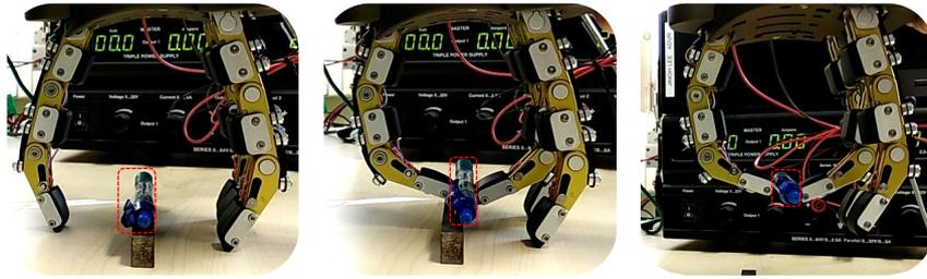
Figure 7: Precisely pinch a pen from table.
