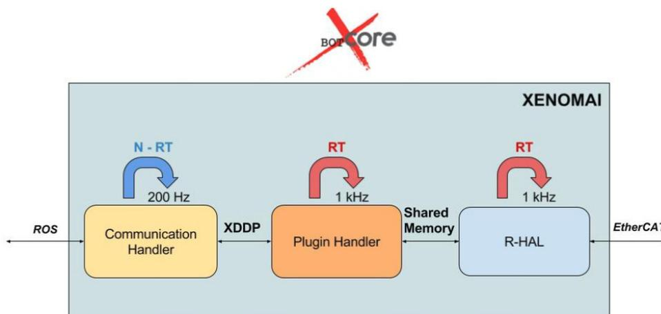
Figure 16: *XBotCore* threads and communication architecture.
