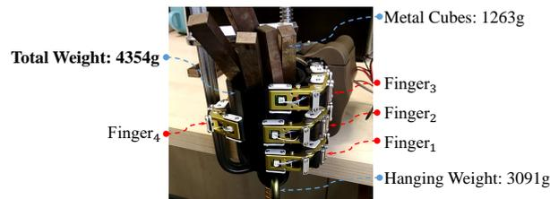
Figure 8: Vertical grasping experiment and finger naming order
