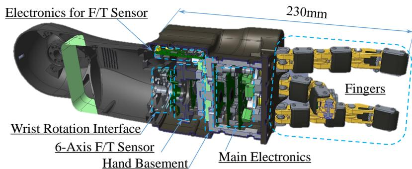
Figure 10: HERI II Hand cross section showing the integration of the various electronics and F/T sensor.
