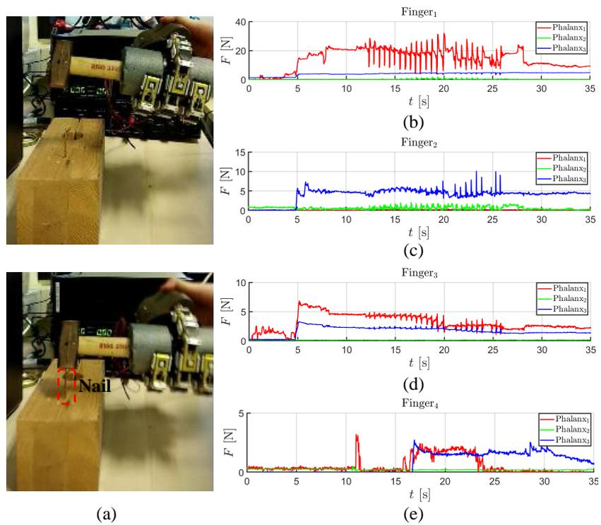
Figure 9: Powerful grasping a hammer during the high impact knocking nail task.
