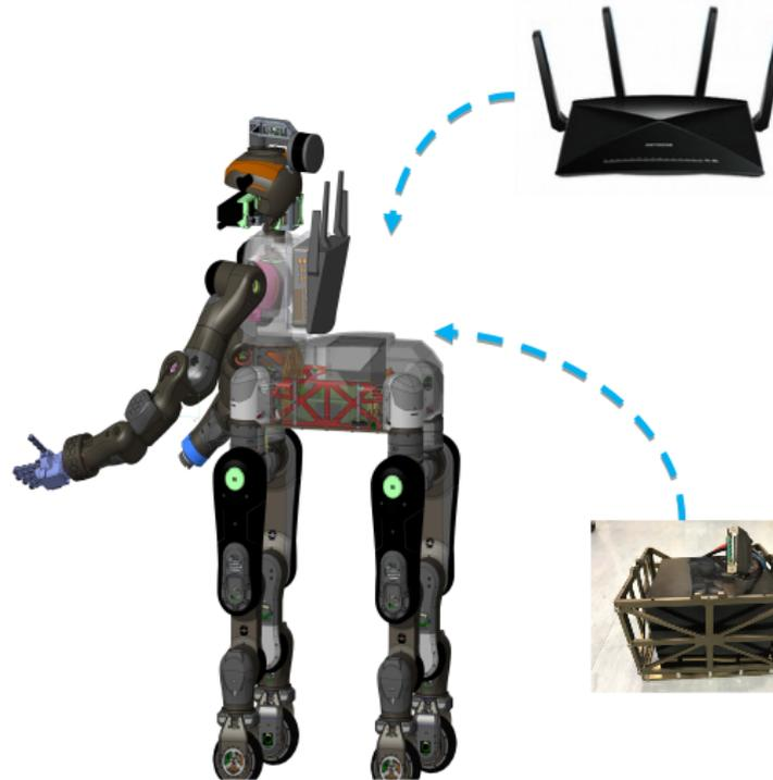
Figure 11: Arrangement of components in the robot trunk.
