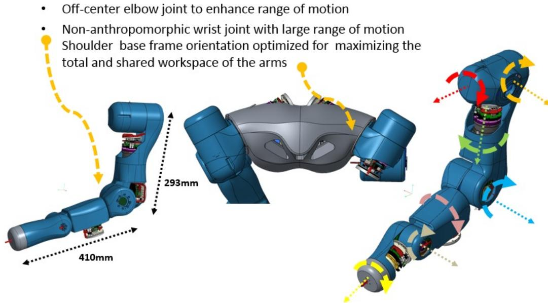
Figure 5: Arm kinematic features.
