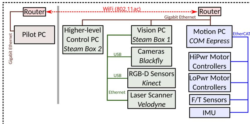
Figure 12: Higher-level schematics of the interconnections of the final CENTAURO robot control and perception components.
