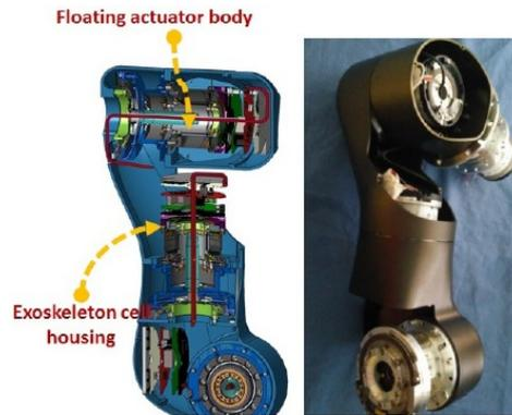
Figure 2: The exoskeleton cell structures and floating body principle.
