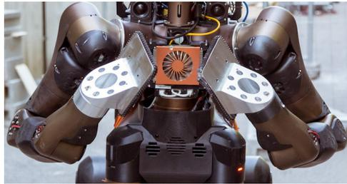
Figure 13: Front-side view of the CENTAURO robot showing the COM Express PC at the torso center (in orange).
