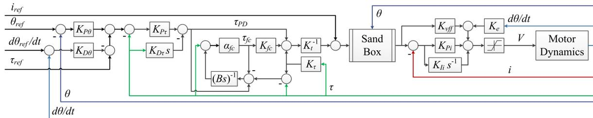
Figure 14: Block diagram scheme of the joint controllers: current feedback in red, torque feedback in green, position and velocity feedbacks in blue.
