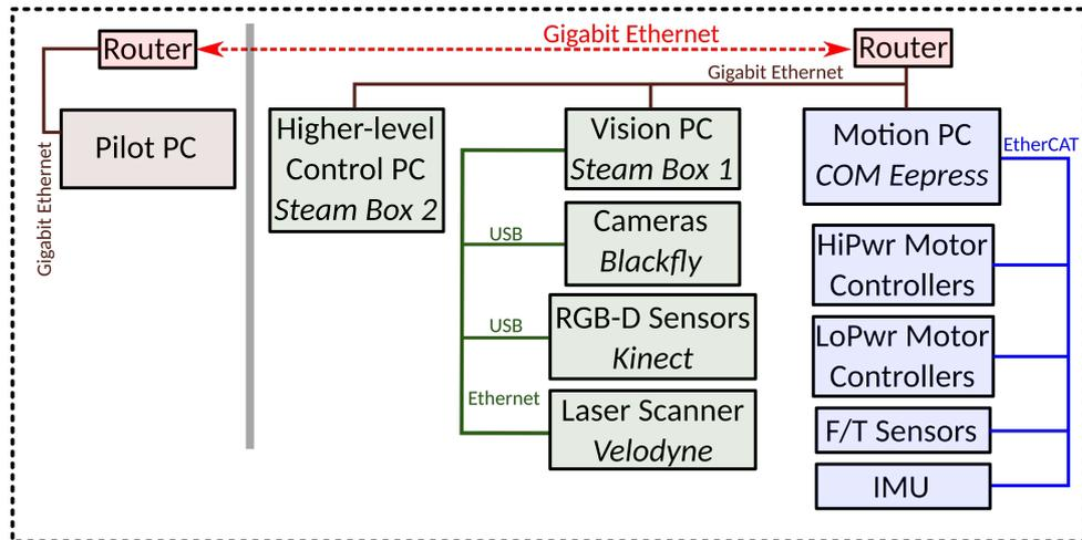
Figure 15: High level schematic of the interconnections of the CENTAURO prototype control, actuation and perception components.
