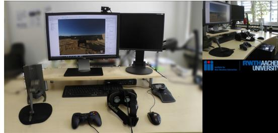
(b) Demonstrator setup - Overview of the devices used with the simulation
