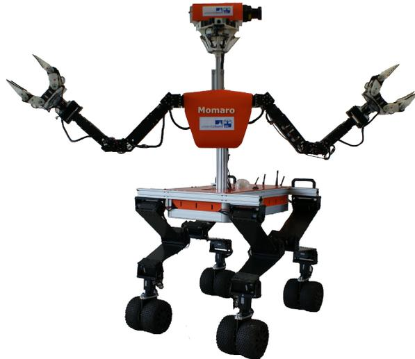
Figure 16: The mobile manipulation robot Momaro.
