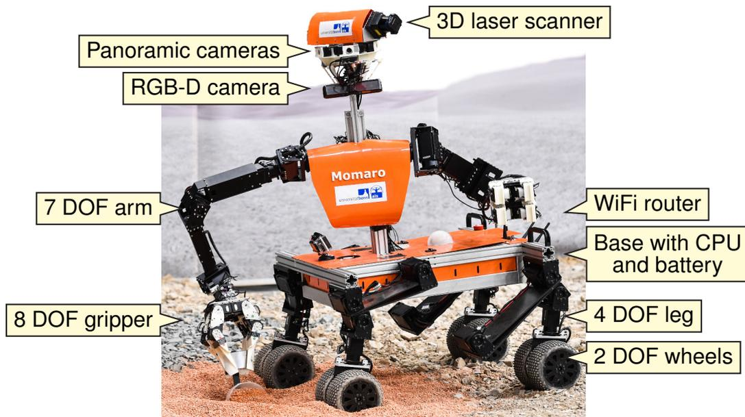
**Figure 1.** The mobile manipulation robot Momaro taking a soil sample.
