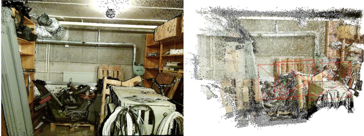
Figure 22: Registration of point clouds in a CENTAURO scenario. Left: some industrial machinery and shelves. Right: A point cloud of the same scene after registration. The camera frustums are outlined in red.
