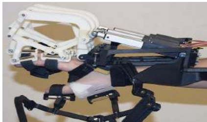
Figure 16: Multi fingered underactuated hand exoskeleton.
