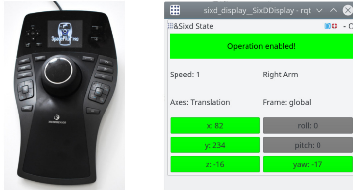
Figure 40: 6D input device (l.) and corresponding GUI (r.) for dexterous wrist control.
