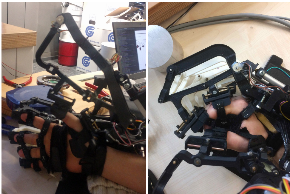
Figure 26: Two different configurations used during ZieglerNichols PI calibration: the hand is completely open (left), the hand is completely closed (right).
