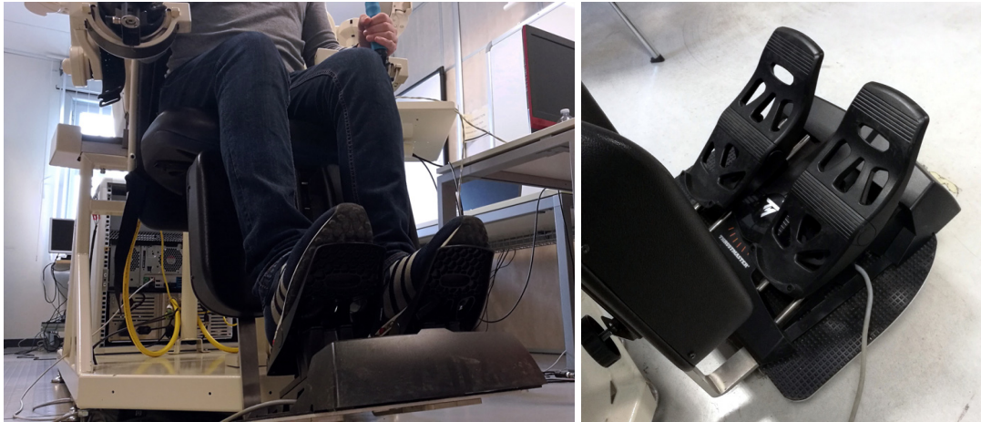
Figure 7: Pedals for controlling the navigation of the Centauro robot integrated in the Control Station
