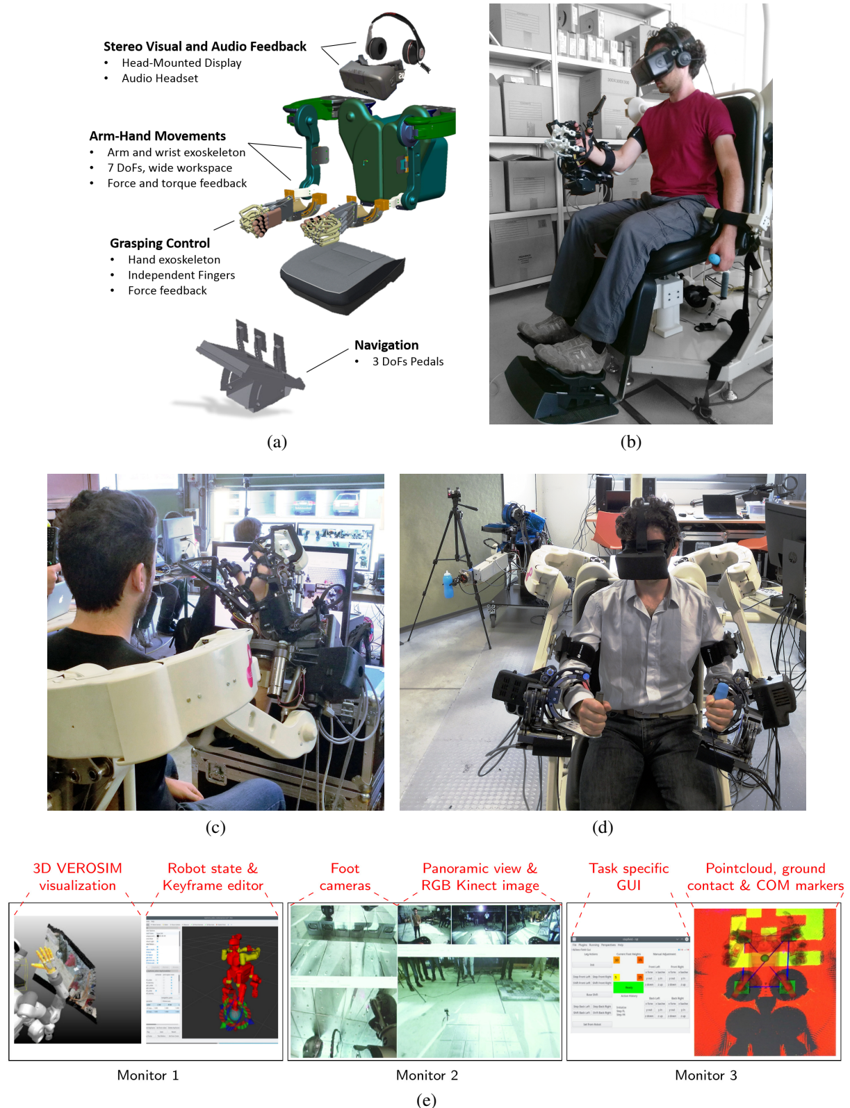
Figure 1: The Centauro Control Station: scheme (a), implementation (b), and application to the Centauro teleoperation scenarios (c),(d). Third person operator interface: environment and robot state visualization(e).
