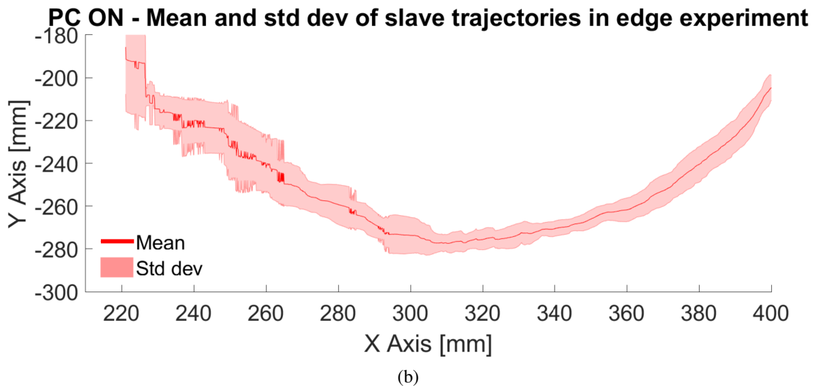
Figure 13: This figure aggregates the slave robot end-effector positions performing the Experiment 1. In (a), mean trajectory with disabled passivity controller, whereas in (b), PC is enabled. The pink area around the mean trajectory represents the standard deviation of the y coordinate for the given x axis coordinate. The larger and more irregular the standard deviation, the more oscillatory is the slave robot.
