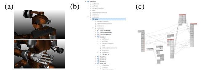
Fig. 7: Representations of the DT: (a) three dimensional view, (b) hierarchical tree of system components (equivalent to an extensible markup language (XML) file), (c) functional flow of data
