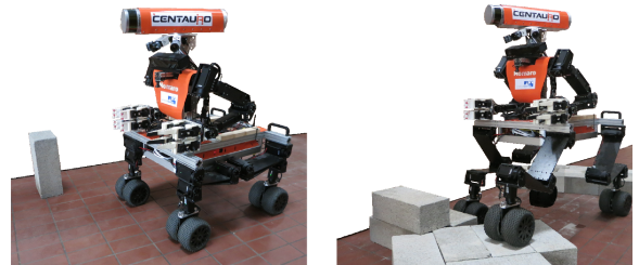
Fig. 1. Our hybrid wheeled-legged mobile manipulation robot Momaro is capable of omnidirectional driving (left) and stepping (right).
