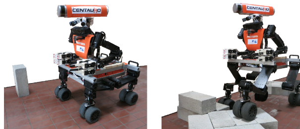
Figure 19: Our hybrid wheeled-legged mobile manipulation robot Momaro is capable of omnidirectional driving (left) and stepping (right).
