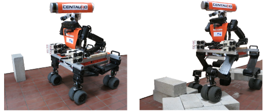
Fig. 2. Our wheeled-legged robot Momaro is capable of omnidirectional driving (left) and stepping (right).
