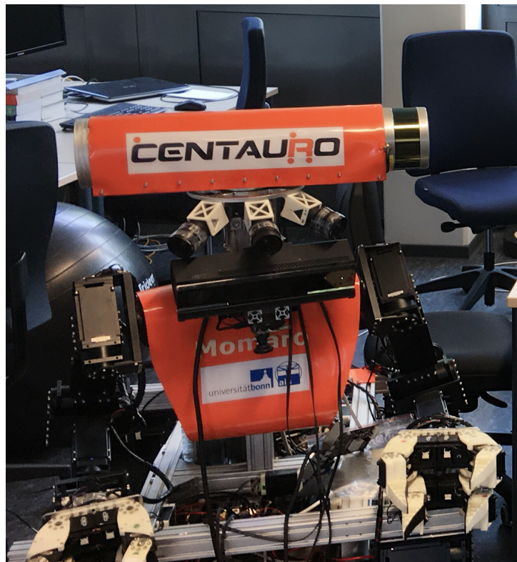
Figure 24: Sensor head of the mobile manipulation robot Momaro, built by UBO. It possesses a rotating Velodyne Puck laser scanner with spherical field of view, a Microsoft Kinect V2 and three Pointgrey cameras. The sensor head setup is similar to the Centauro sensor head.
