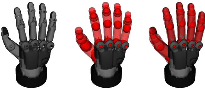
Figure 6: Visual and collision model of the robotic hand. At rightmost both models are displayed simultaneously to show the goodness of the capsule approximation.
