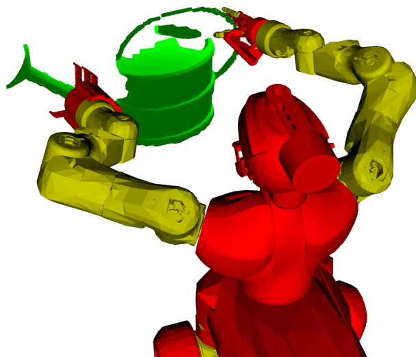
Figure 1: Pre-grasp pose of the Centauro robot for dual-arm grasping of an unknown watering can.
