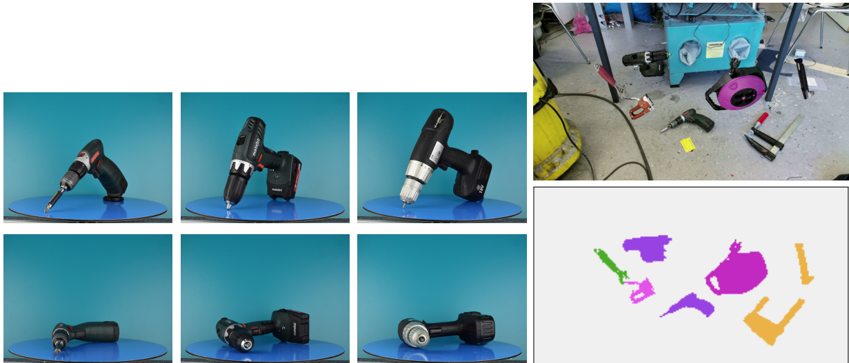
Figure 18: Turntable capture and scene synthesis. Left: Different drills on the turntable as captured by a DSLR camera. Right: Synthetic training scene generated by inserting new objects. The top image shows the resulting color image, the bottom shows generated ground truth for training the segmentation.
