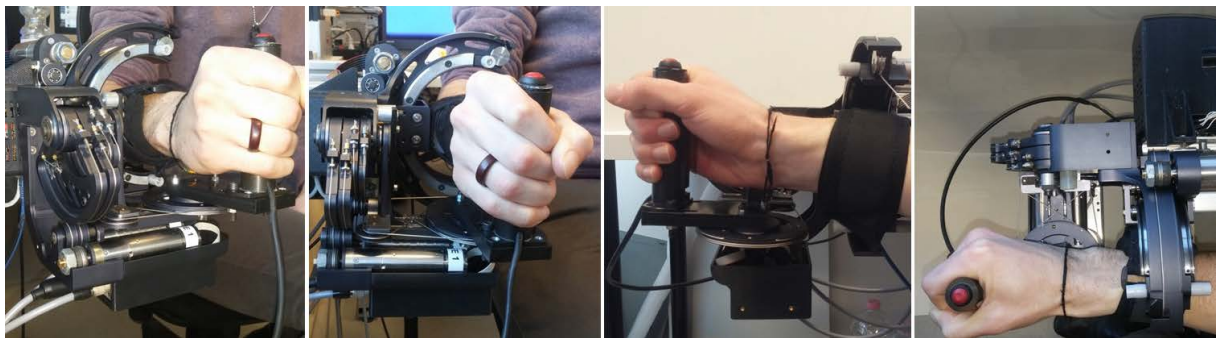
Figure 12: The wrist exoskeleton worn by an operator. Left: Isolated test. Right: Mounted on the arm exoskeleton.
