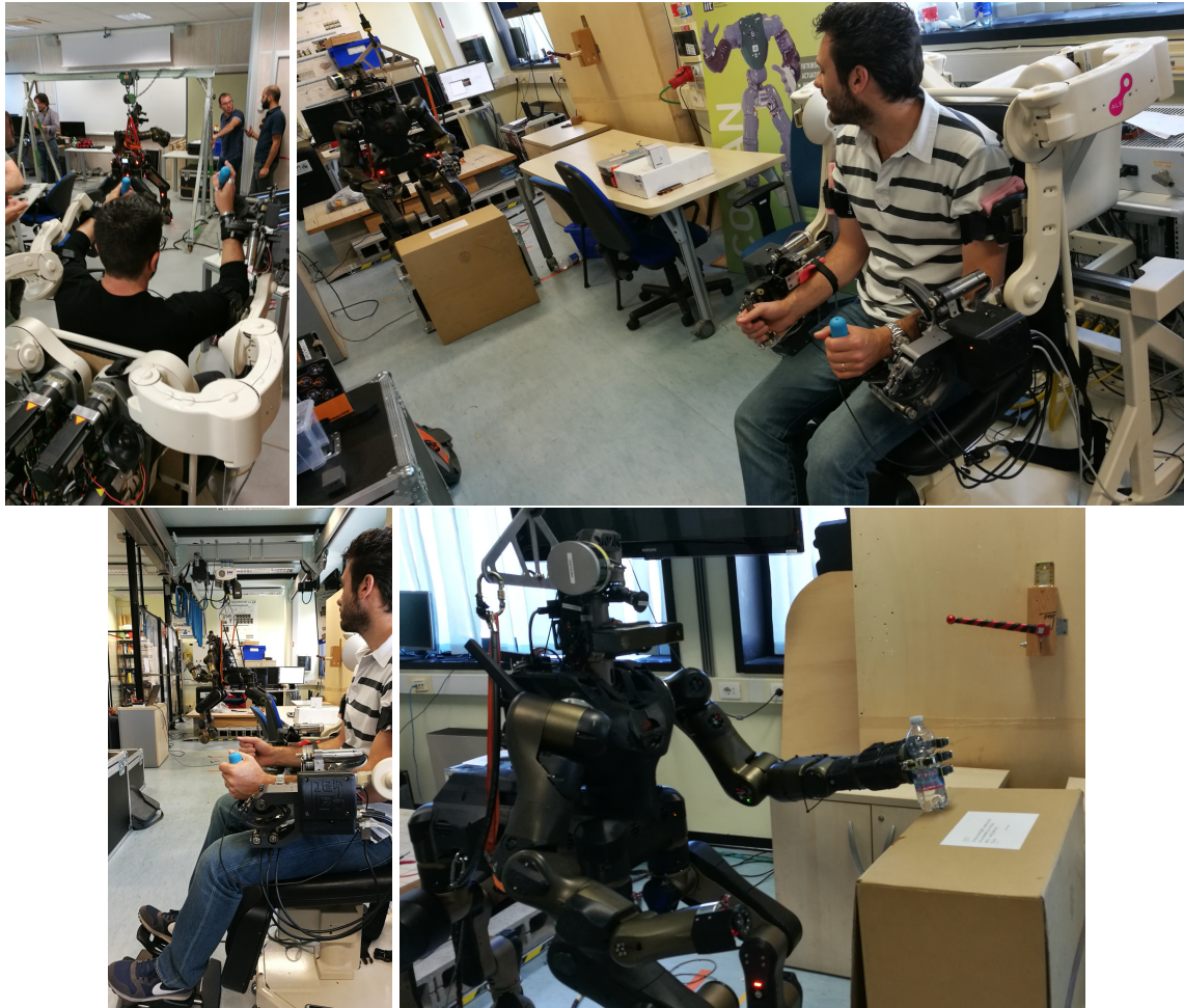
Figure 16: Test and tuning of arm teleoperation (workspace, offsets, force feedback parameters) between the HandExos, the Schunk Hand and the HERI Hand.
