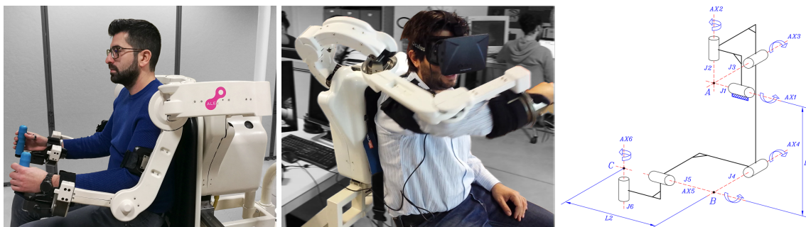
Figure 10: The bilateral arm exoskeleton module, featuring four actuated DoFs (shoulder and elbow) in a wide operative workspace.
