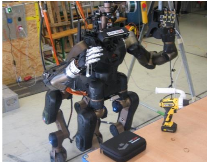
Figure 16: Centauro in front of the two-handed driller which it was to grasp autonomously.
