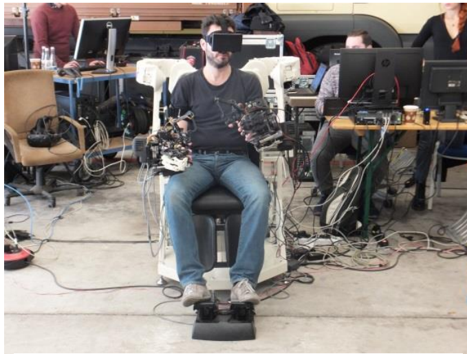
Figure 1: The Full-body Telepresence suit.
