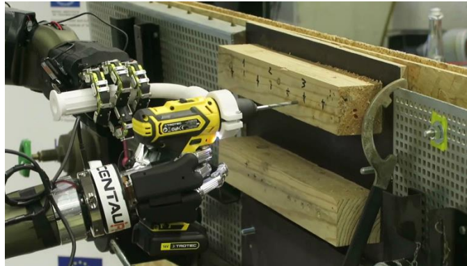
Figure 13: Centauro approaching the wooden block with the driller tip.
