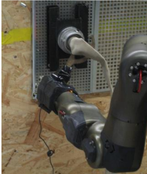
Figure 9: Centauro using a special tool to fasten the fire hose to the nozzle.
