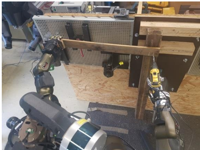
Figure 12: Centauro screwing a screw to fix a wooden board to a wooden block.
