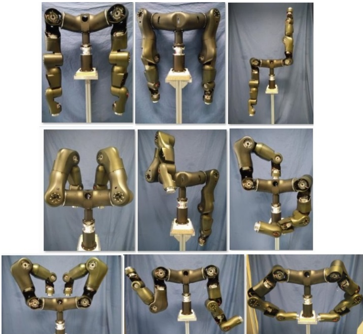
Figure 18: D2.2 demonstrator showing CENTAURO upper body prototype in different arm poses.
