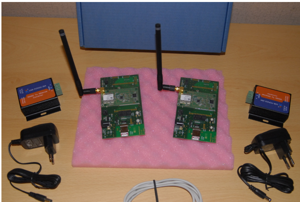
Figure 5: Amber Wireless link AMB8636.
